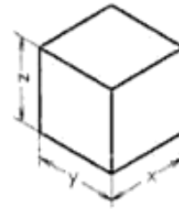
Fig. 16.10 Dimensioning of isometric drawings.
